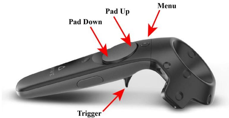
Pressing the Menu button switches the controller between MOVE and PULL mode.
