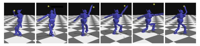
Fig. 5. Reaching a moving target, stepping when necessary. A sequence of frames of full body motion synthesized in real-time for the HRP2 robot. The robot is trying to reach the moving target while stabilizing itself. When the rotation causes the legs to collide, the robot stumbles, takes a step to balance itself, and reaches for the target once more.
