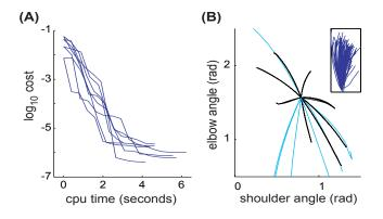
Fig. 5. (A) Cost over iterations of ILQG. (B) Hand paths for random initial conrol laws (inset) and optimized paths (black) to 8 targets. Poor local minima (7 out of 80) are shown in cyan.
