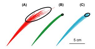
Fig. 4. Effects of control-dependent noise on hand reaching trajectories, under different control laws. (A) open-loop control; (B) closed-loop control; (C) closed-loop controller optimized for deterministic system.
